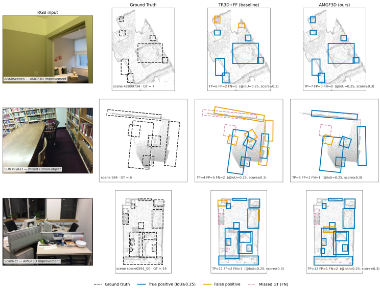
Figure 5: Qualitative comparison on ARKitScenes, SUN RGB-D, and ScanNet. Columns: paired RGB frame, bird’s-eye view ground truth, TR3D+FF, and AMGF3D. Box colors denote TP/FP/FN at \text{IoU} \geq 0.25 . On ScanNet and ARKitScenes, the single posed RGB frame covers only part of the reconstructed scene, and the BEV is cropped for legibility. AMGF3D recovers small or partially observed objects and removes baseline false positives.
